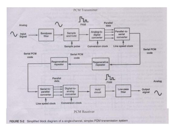
In the receiver, the *serial-to-parallel converter* converts serial pulses received from the transmission line to parallel PCM codes. The *digital-to-analog converter* (DAC) converts the parallel PCM codes to multilevel PAM signals. The hold circuit is basically a low pass filter that converts the PAM signals back to its original analog form.
