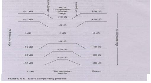
Figure 5-9 illustrates the process of companding. An analog input signal with a dynamic range of 50dB is compressed to 25 dB prior to transmission and then in the receiver expanded back to its original dynamic range of 50 dB. With PCM, companding may be accomplished using analog or digital techniques. Early PCM Systems used analog companding, whereas more modern systems use digital companding.
